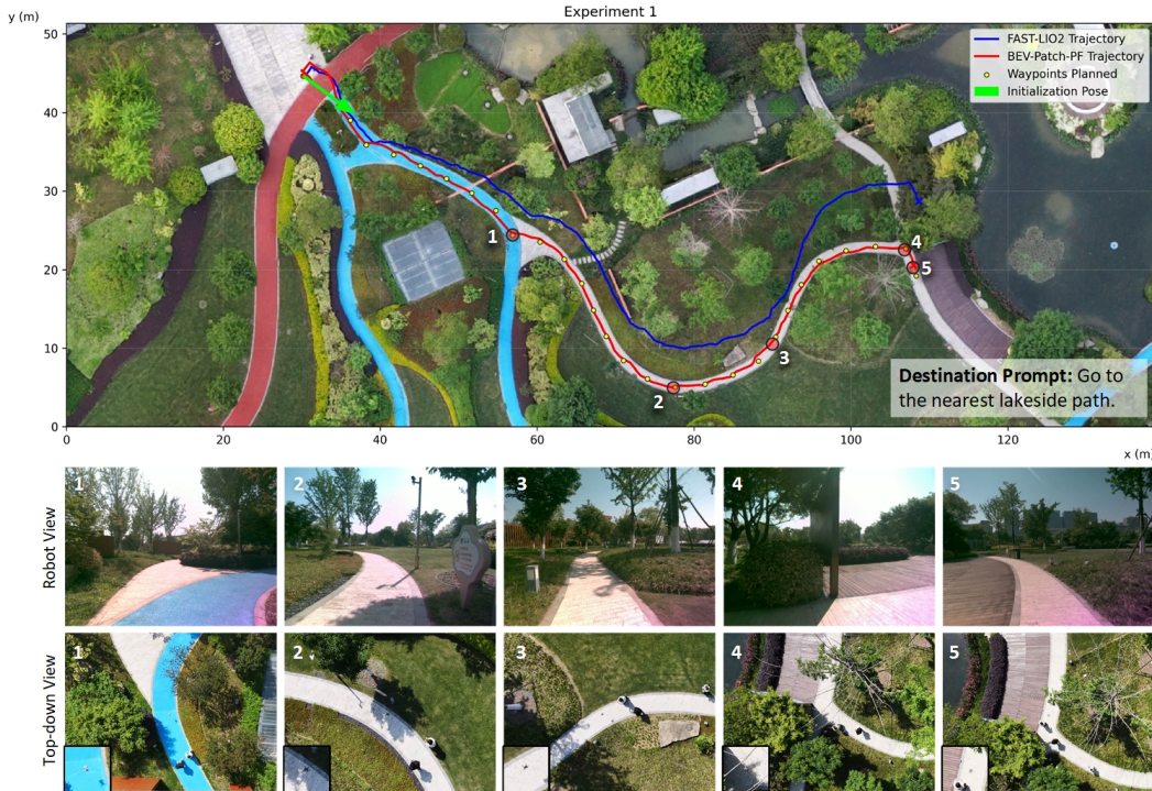
Figure 6: Experiment 1. Navigation in a park. The initial global pose estimate contains relatively large errors, making FAST-LIO2 alone insufficient for long-range navigation.
