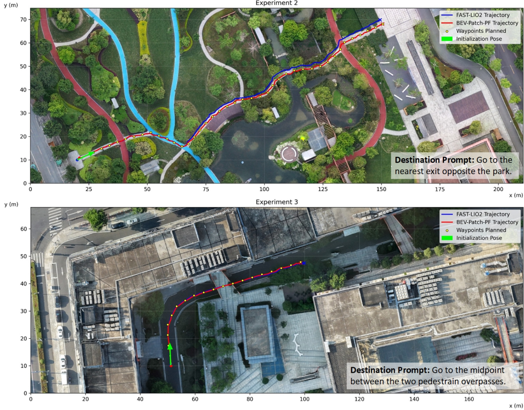
Figure 7: Experiment 2: Navigation in a park. Even with an accurate initial pose, unacceptable drift occurs during long-range navigation. Experiment 3: Navigation in structurally complex buildings.
